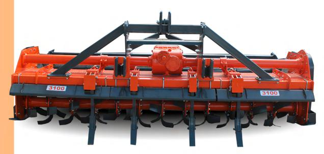
**Rotovator:** It is a soil cultivation machine that mixes the soil from the bottom to the surface with the help of horizontally rotating hoes. It is used to prepare the seed bed, aerate the soil, and ensure that plant waste and weeds are broken down and completely mixed into the soil. While the machine is running, the roller levels the soil
